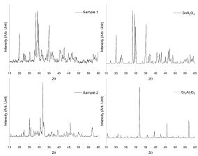
The XRD pattern of two samples already synthesized by MASS. The sample 1 matches with the structure of  $SrAl_2O_4$  phase (ICSD Code#160296) and the sample 2 matches with the structure of  $Sr_3Al_2O_6$  phase (ICSD Code#66062), despite having an additional peak at  $2\theta$ =25° attributed to impurities in the sample.
